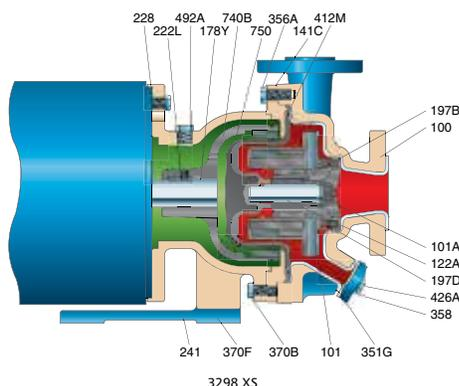
The 3298 S provides additional low flow coverage below the hydraulics of the smallest traditional ANSI pump size. XS pumps meet user requirements for low flow capabilities. Applying an oversized ANSI pump is not required.
